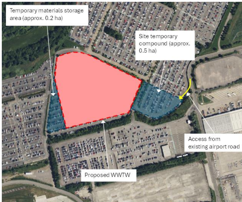
Figure 61: Temporary Construction Compounds associated with the On-airport WWTW
