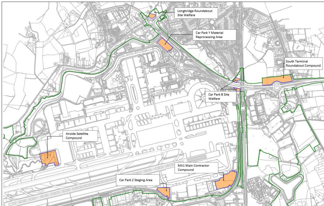
Figure 5: Anticipated locations of temporary construction compounds
